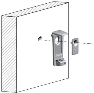
Recommended fixing countersunk screw type - head Ø 4 mm max.
