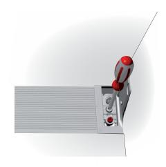
The slim side bracket makes the use of tools very easy and comfortable as there is plenty of space between the side and the screwdriver.
