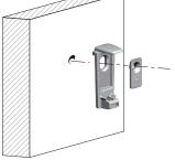
Recommended fixing countersunk screw type - head Ø 4 mm max.
