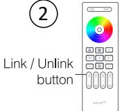
Short press "I" button 5 times within 3 seconds when light on
